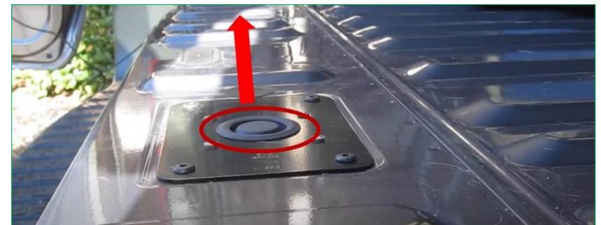
"Removal of the grommet"
