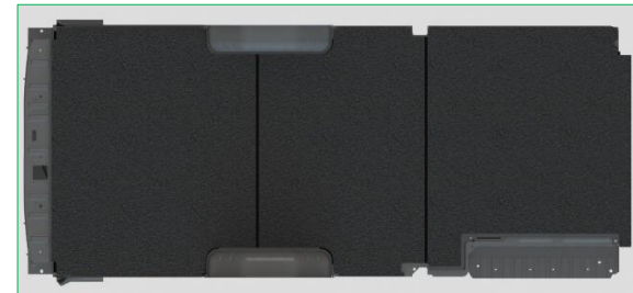
"View of Floor Piece A, H1, Floor Piece C, H2 and Floor Piece E installed in the vehicle"
