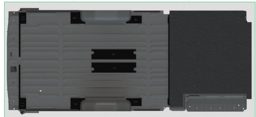
"Positioning of combined set of 'Floor Piece A and H1' in the vehicle"
