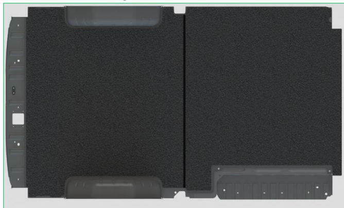
“View of Floor Piece A, H1 and Floor Piece B installed in the vehicle”
